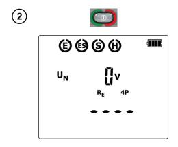
Turn on the meter using **ON/OFF** button.
