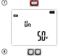
Use **UP** and **DOWN** buttons to set the measuring voltage at 25 V or 50 V. The measuring voltage set relates to all measurement functions in the meter.
