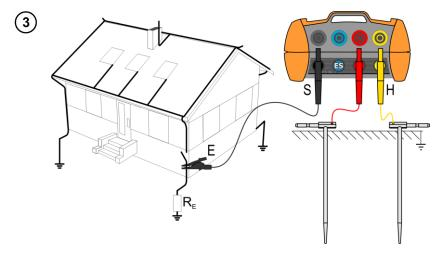
Test leads should be connected to the measurement terminals in the device, as shown above.
