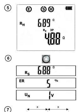
After completing the measurement, results are displayed for all the measurements carried-out: at the bottom of the screen, the main result is shown for  $R_E$ , whereas the upper part of the screen shows additional results for  $R_H$ . The result is displayed for 20 seconds. The result can be recalled by pressing UP button.
