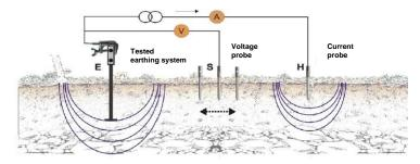
The scheme of measuring the earthing resistance with the 'technical method' is shown above. The figure shows the measurement of earthing resistance  $R_E$ . To perform the measurement, use two additional auxiliary electrodes:
