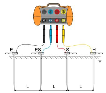
Connect the four aligned and equally spaced auxiliary electrodes, which are driven into the ground, to the meter, and do so in accordance with the diagram above.
