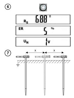
Use **UP** button to view the component results in the following order:  $R_H \rightarrow R_S \rightarrow ER \rightarrow U_N$ , where:
