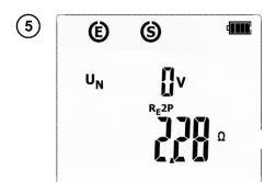
After the measurement, its result is shown: at the bottom of the screen, the main result is shown for  $R_E 2P$ , whereas the upper part of the screen shows the measured interference voltage  $U_N$ . The result is displayed for 20 seconds. The result can be recalled by pressing UP button.
