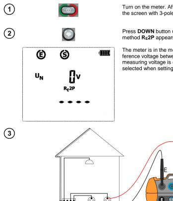
Turn on the meter. After turning the meter ON, the screen with 3-pole method  $R_E 3P$  is shown.
